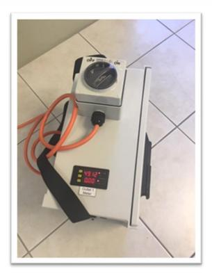
LINK N LIGHT can be powered by a 150W (will power 15 metres) or a 600W (will power 45metres) Power Supply Enclosure. The PVC Power Supply Enclosure weights just over 10kg. it comes with a tool bag type shoulder strap, has a main isolator, power meter and outlet plug. All protection for the incoming and outgoing circuits are inside the enclosure.
